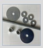
1/4 Inch threaded rod (less than 8 inches needed), (4) 1/4 inch stainless steel washers, (2) 1/4 inch stainless lock nuts and (2) 1/4 inch fender washers (optional) to act as trim to cover the bearings. I painted my fender washers with a brass colored paint to match the rods.
