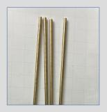
(16) ¼ inch brass rods are needed for the windmill, 8 for each spinning wheel. My sculpture used 14 inch rods though in hindsight, 12 inch or 10 inch rods might have worked better to reduce the overall width of the sculpture.
