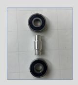
(4) Roller blade bearings and (2) Roller blade bearing spacers are needed for the rotational hubs. One set of bearings and spacer will fit tightly in the middle of each windmill hub. See the video for more detail on assembly.
