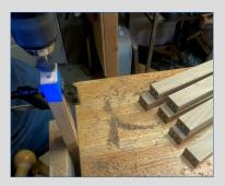
Matching the hole drill pattern used above, create another small jig to center the drill holes in both ends of each stave – 4 on each leg, 8 staves total. Each stave will then accommodate a 1  $\frac{1}{2}$  inch long oak dowel at  $\frac{1}{4}$  inch thick.
