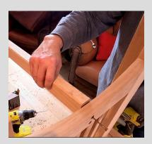
The trestle board is finally attached to the center of each arched bottom frame piece with (2) 3 inch heavier duty screws. These were counter sunk with a Forstner bit to leave a clean, circular hole, and those holes provide a way to trim out the trestle attachment with trim dowels, or like you saw in the video, I created an end cap to cover the screws.
