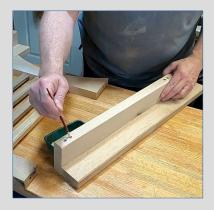
Once the center stave section is dry, you can complete each leg structure by gluing in the thicker 3/8 inch dowels into the vertical legs, and then glue the leg pieces into the center stave assembly. Clamp them together checking the full assembly for square, and wipe off any excess glue with soapy water.
