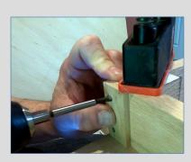
Assemble the underside table apron by squaring the corners of the apron frame pieces and drilling in holes for ¼ inch oak dowels. The 31 ½ inch shorter pieces should face outward towards each end of the table, showing the dowel detail as seen with the legs. A small template measured out to center the holes will help consistency of your drill pattern.
