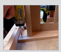
The flat panel on the top of each leg gives you some flexibility as to where the leg is positioned on the underside of the table. For me, I needed enough distance between the legs to accommodate 3 of our dining chairs, so the distance between the inside edges of my legs is 43 inches. The flat oak top plate is then drilled and screwed into place with 1 ½ inch cabinet screws.
