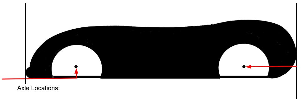
For both wheels on both sides, the center point for the wheel well cut out and for the wooden axle drill hole is the same when measured from the front or back of the block, and then from the bottom of the block.
